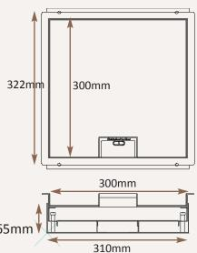
Stainless steel. Lid recess made to suit floor covering Outlet plate options Fits 3 standard outlet plates.
