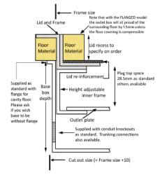
Frame size 320x250mm with 12.5mm visible trim flange Base box size 330x260mm
