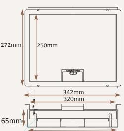
Lid option -Stainless steel. Lid recess made to suit floor covering Outlet plate options Fits 3 standard
