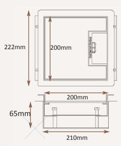
Frame size 200x200mm with 12.5mm visible flange
