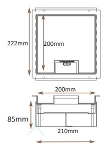
Frame size 200x200mm with 12.5mm visible trim flange Base box size 210x210mm  $\,$
