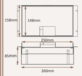
Lid option -Brushed brass. Lid recess made to suit floor covering Outlet plate options Fits 1 standard outlet plate.
