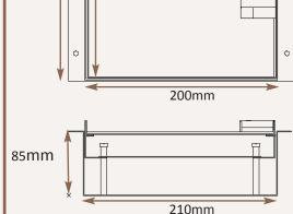
Frame size 200x200mm Base box size 210x210mm
