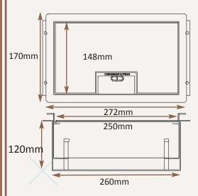
Frame size 250x148mm (with 12.5mm overall visible flange) Base box size 260x158mm Lid recess - advise on order to suit floor covering
