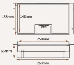
Lid option -Brass. Lid recess made to suit floor covering Outlet plate options Fits 1 standard outlet plate.
