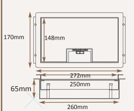
Lid option -Stainless steel. Lid recess made to suit floor covering Outlet plate options Fits 1 standard outlet plate.
