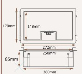
Lid option -Stainless steel. Lid recess made to suit floor covering Outlet plate options Fits 1 standard outlet plate.
