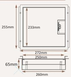
Frame size 233x250mm (with 12.5mm overall visible flange) Base box size 243x260mm Lid recess - advise on order to suit floor covering Base with 20 & 25mm conduit knockouts in base and sides
