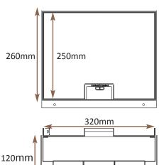
Frame size 320x250mm Base box size 330x260mm Lid recess - advise on order to suit floor covering Base with 20 & 25mm conduit knockouts in base and sides
