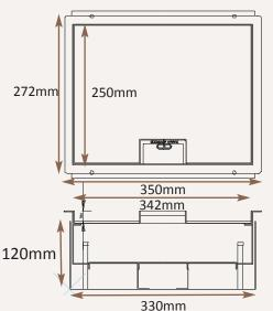
Frame size 320x250mm (with 12.5mm overall visible flange) Base box size 330x260mm Lid recess - advise on order to suit floor covering Base with 20 & 25mm conduit knockouts in base and sides
