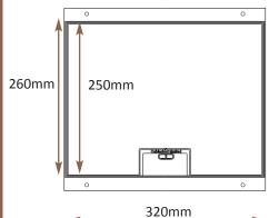
Lid option -Brass. Lid recess made to suit floor covering Outlet plate options Fits 3 standard outlet plates.
