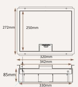
Frame size 320x250mm (with 12.5mm overall visible flange) Base box size 330x260mm Lid recess - advise on order to suit floor covering
