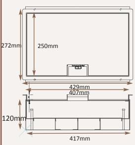
Frame size 407x250mm (with 12.5mm visible trim flange) Base box size 417x260mm
