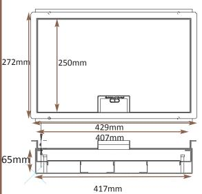
Frame size 407x250mm (plus visible trim flange 12.5mm) Base box size 417x260mm Lid recess - advise on order to suit floor covering Base with 20 & 25mm conduit knockouts in base and sides
