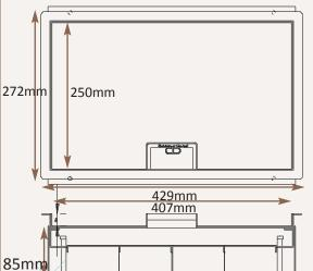
Frame size 407x250mm (with 12.5mm visible trim flange) Base box size 417x260mm Lid recess - advise on order to suit floor covering Base with 20 & 25mm conduit knockouts in base and sides
