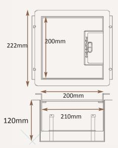
Frame size 200x200mm with 12.5mm visible flange
