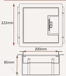
Frame size 200x200mm with 12.5mm visible flange
