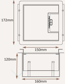
Frame size 150x150mm (with 12.5mm visible trim flange) Base box size 160x160mm Lid recess - advise on order to suit floor covering
